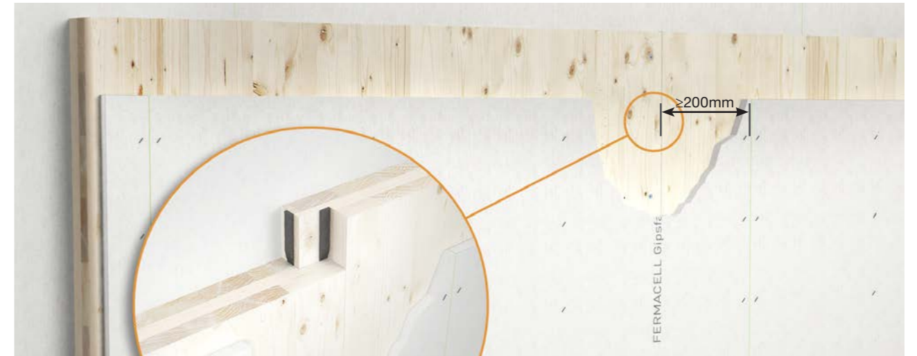
CLT element joint - step joint connection
